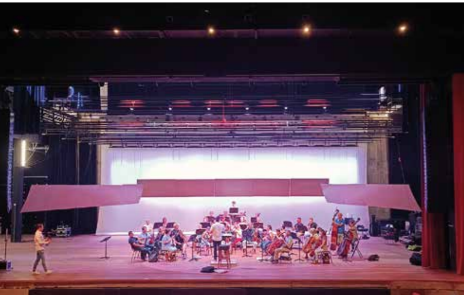
Above: Acoustic tests for fine-tuning the stage acoustics in Theater De Oranjerie, Roermond, with musician members of Kahle Acoustics and then with the orchestra
