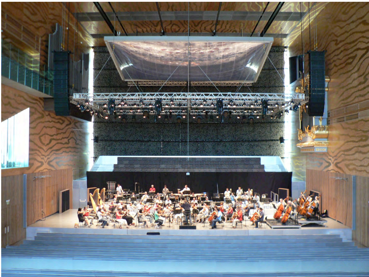
Concert Hall Casa da Música during the acoustic tests: rear wall absorption, raised and tilted canopy.
