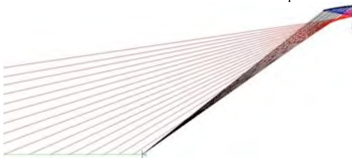
Acoustic simulation of a second order reflector: black rays shape the direct wave towards the vertical curved surface; red rays shape the reflected wave (after two successive reflections). The green line shows the area covered with reflections.
