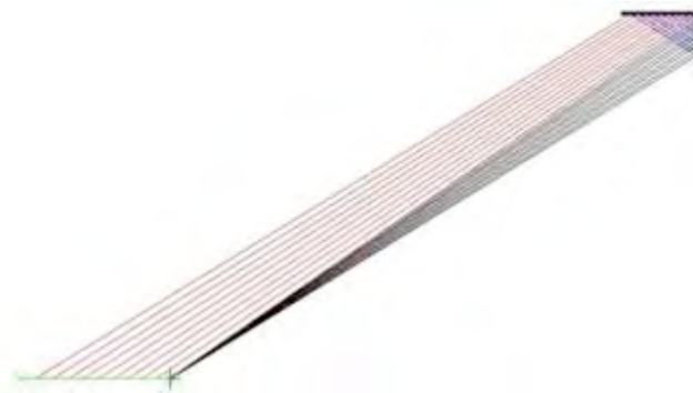
Acoustic simulation of a second order reflector: black rays shape the direct wave towards the vertical surface (for clarity the paths towards the horizontal surface has not been drawn), red rays shape the reflected wave (after two successive reflections). The green line shows the area covered with reflections.
